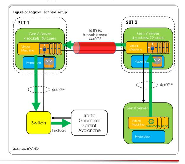
The two systems under test were both four-socket, 4 RU HPE ProLiant devices: the DL580 Gen9 and Gen8 running the 6WIND Turbo IPsec software (34 cores) and 6WIND Virtual Accelerator in the hypervisor (24 cores). The rest of the system components under test are as follows:
